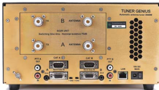
Figure 1 — FlexRadio Tuner Genius XL rear panel (SO2R version).
