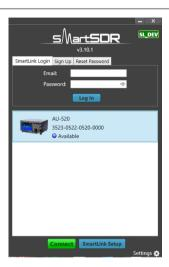
To start SmartSDR, double click the radio in the Radios area of the dialog box or click the radio once and then press the CONNECT button that appears at the bottom of the screen. "Available" indicates that you may connect to the radio.
