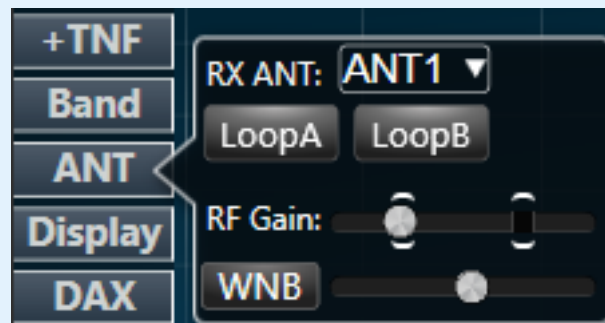
Figure 137: Slice RX antenna and WNB controls
