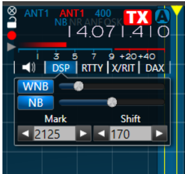
Figure 163: Slice RTTY WNB NB mark shift controls
