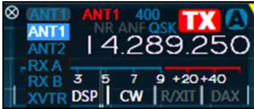
Figure 132: Slice antenna dropdown ANT1 ANT2 RX XVTR
