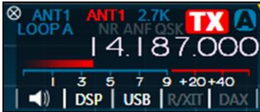
Figure 134: Slice with LoopA antenna selected
