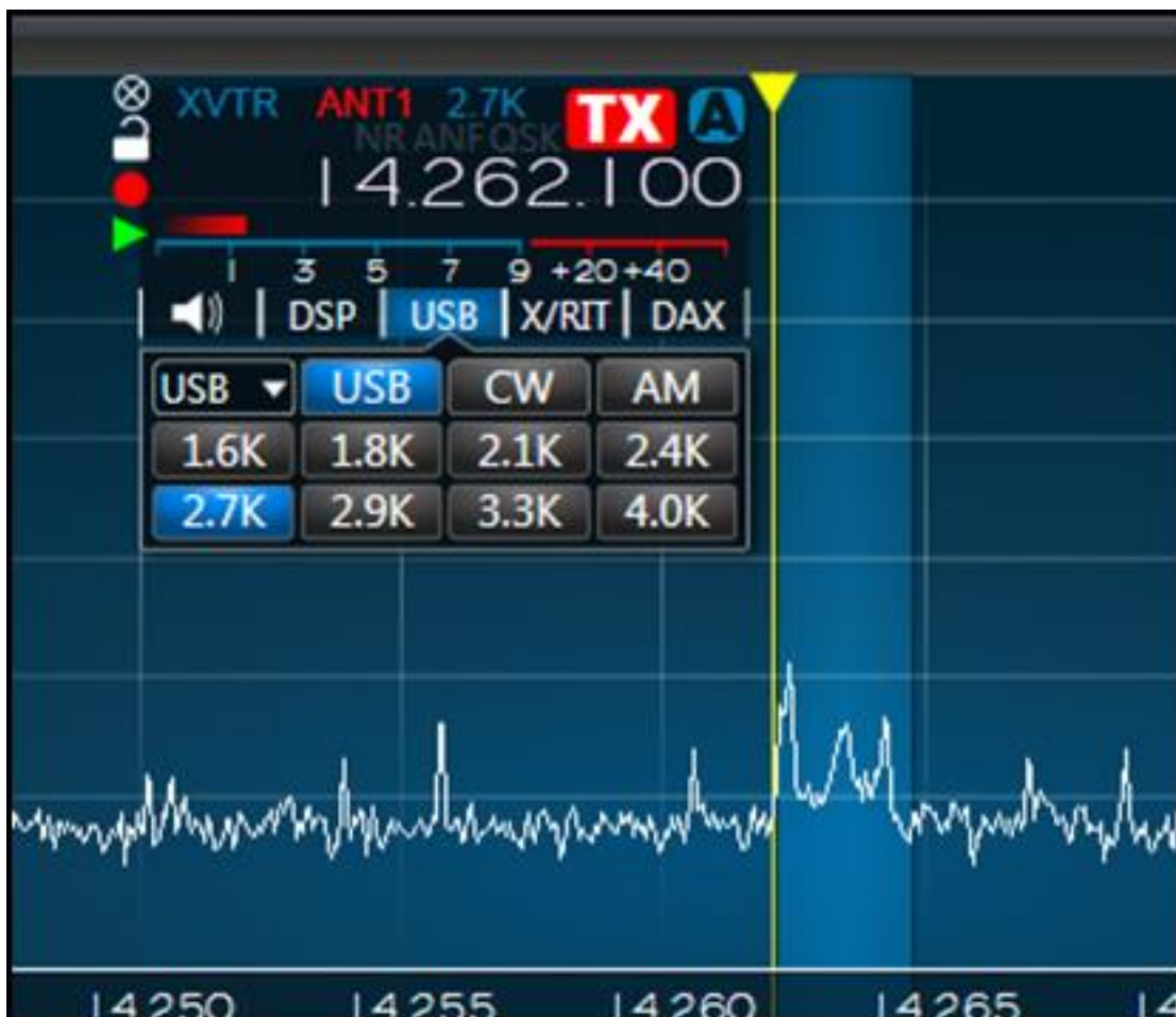
Figure 97: USB slice panel with panadapter waterfall
