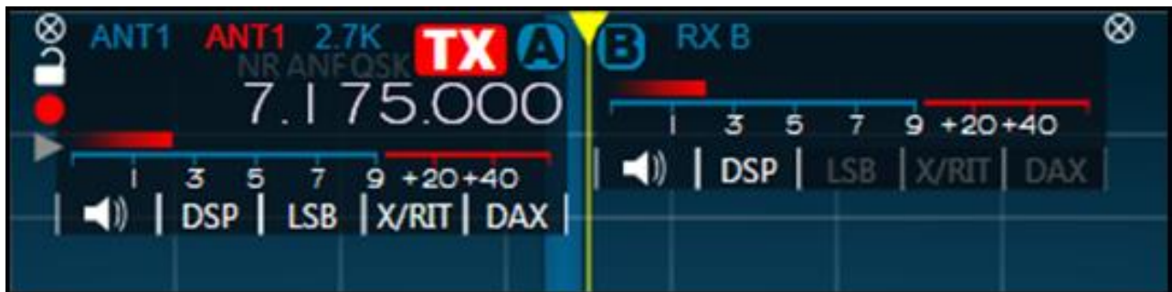
Figure 120: Diversity slice A and RX B panel
