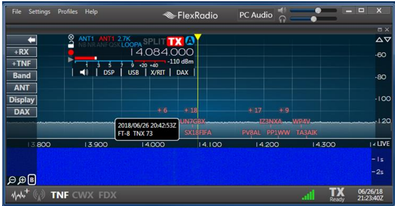
Figure 144: Main window spots with TNF tooltip
