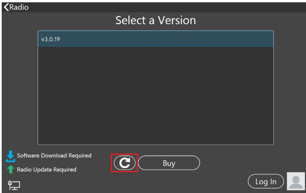
When the license is updated, the refresh button will disappear and the Buy button will change to a Run button. Tap the Run button to connect SmartSDR v3 for an M Model FLEX-6000 or Maestro to your FLEX-6000.
