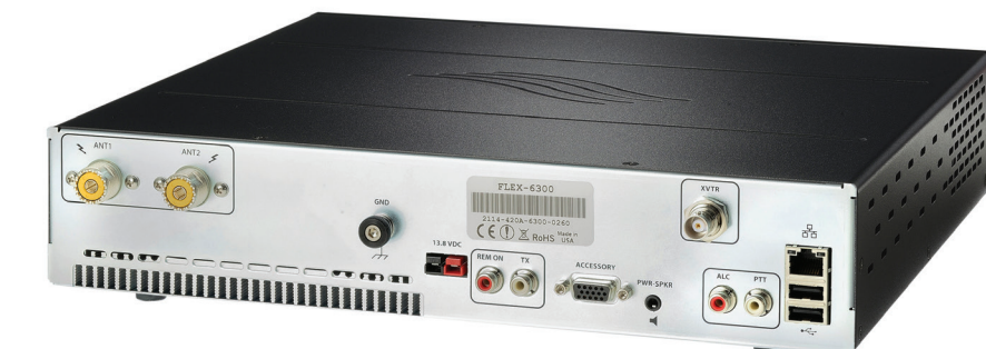
Figure 9 — The FLEX-6300 rear panel. The transceiver has two antenna ports, a transverter jack, amplifier key and ALC jacks, and an Ethernet jack for connection to the PC.
