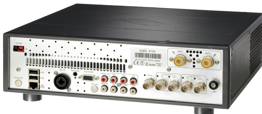
Figure 10 — The FLEX-6700 rear panel. Some of the available connections include two antenna ports, separate receive antenna connections for each SCU, four transmit relay outputs, amplifier ALC, line/mic inputs, connections for an external reference oscillator, and an Ethernet jack for connection to the PC.
