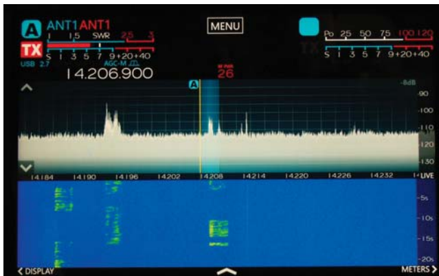
Figure 4 — A screenshot of the FLEX-6400M display showing a single panadapter display, with waterfall below, including the frequency tuned by VFO A.
