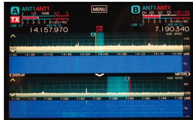
Figure 5 — Same as in Figure 4, except a second spectrum and waterfall display are added below the first. Note that the second is on a different band, bandwidth, and mode. Either can be anywhere within the FLEX-6400M's tuning range, but both must be from the same antenna.
