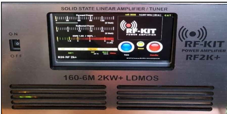
The new B26-RF2K+ amplifier now interfaces with the Flex 6600M in WØAD's station
