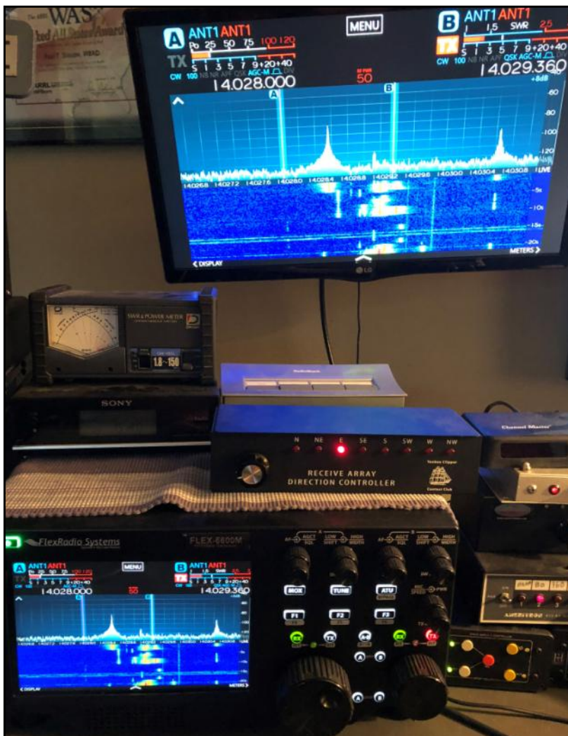
The Flex 6600M has an HDMI Port allowing the radio front panel to be displayed on an external monitor
