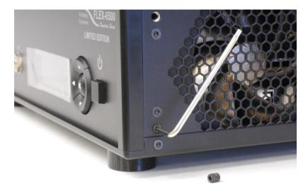
Remove the Set screws on the left side of the radio at this time.
