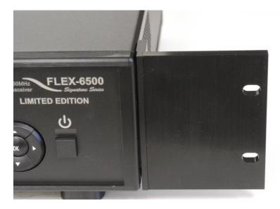
Insert the two (2) Phillips screws as shown in the image below (handle option shown in image) to secure the Rack Mounting bracket to the FLEX-6000. Screw the Phillips screws in securely but do **not** over tighten making certain not to cross thread the screws.
