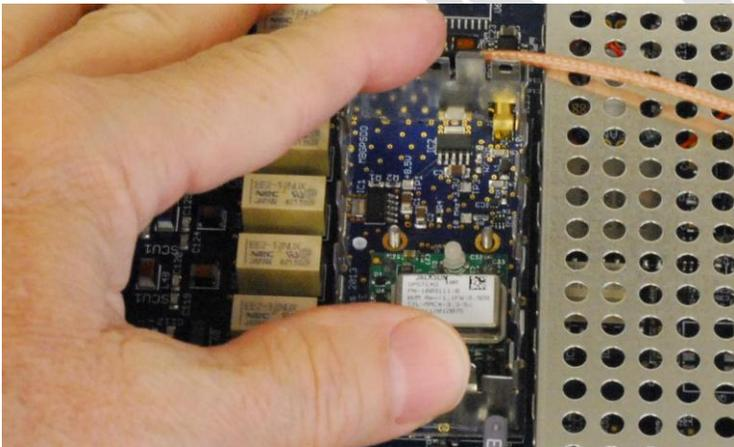
Carefully thread a 5/32" (4mm) spacer onto each threaded stud making sure not to cross thread the stud as shown in the image below.
