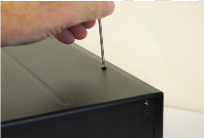
Using the long portion of the “L” TORX wrench install the three (3) short **Bottom Cover Side screws** on the **left** side of the FLEX-6000. Then install the remaining three (3) short Bottom Cover Side screws on the **right** side of the FLEX-6000. The image below shows the installation of the left side bottom Cover Side screws.
