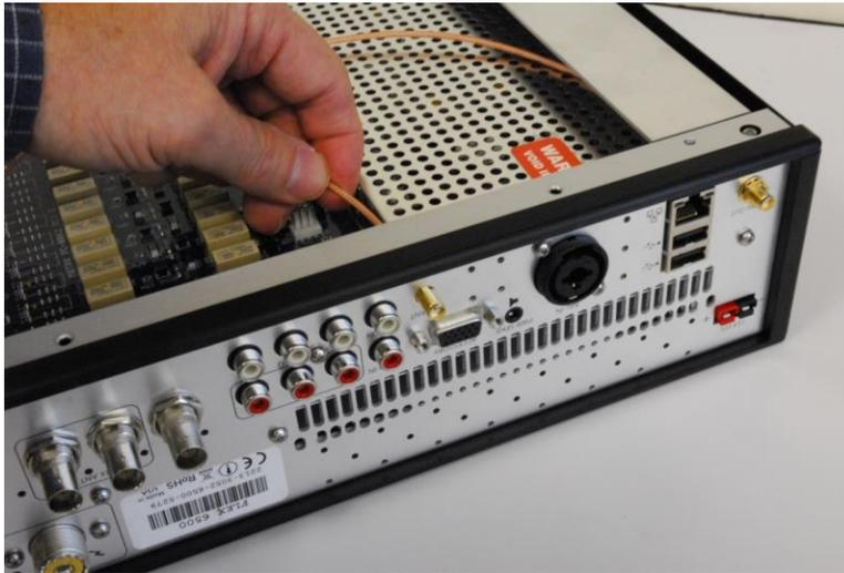
While firmly holding the cable assembly in place with one hand, insert the lock washer on the threaded SMA connector. Carefully install the SMA connector 5/16" (8 mm) hex nut on the threaded SMA connector being careful not to cross thread the SMA connector. Tighten hex nut with your fingers so that the coax cable assembly will freely rotate.
