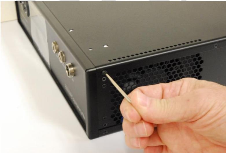
After removing the bottom cover side screws remove the six (6) stainless steel (silver) **Bottom Cover screws** using the long portion of the “L” TORX wrench. Retain the bottom Cover screws for re-installation. The image below shows the removal of the Bottom Cover screws.
