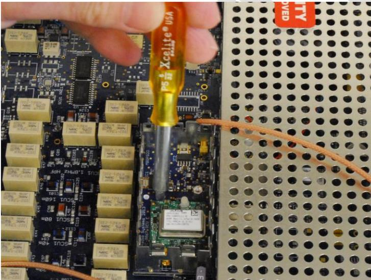
Press the **10MHZ OUT** coax assembly onto the MMCX connector on the GPSDO assembly module that faces the *front* of the FLEX-6000 as shown below.
