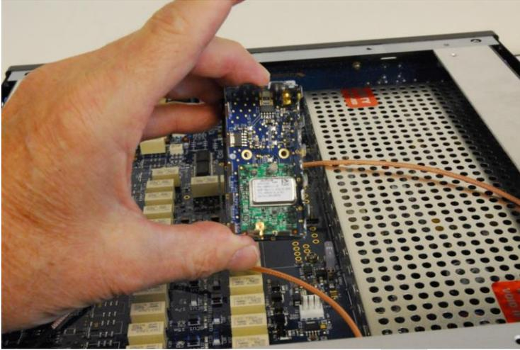
Insert the GPSDO module assembly onto the PC board so that the two (2) threaded screw studs are visible inside the GPSDO assembly as shown below. When oriented correctly, press down firmly to properly seat the GPSDO assembly module.
