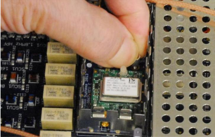
Using a 5/32" (4mm) socket wrench or nut driver gently tighten the spacers on the threaded stud to firmly attach the GPSDO assembly module to the PC board. *Do not over tighten the threaded spacer.*
