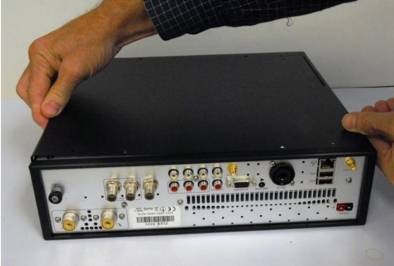
After reinstalling the bottom cover install the six (6) stainless steel (silver) **Bottom Cover screws** using the long portion of the "L" TORX wrench. The image below shows the installation of the Bottom Cover screws.
