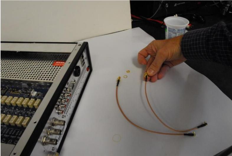
Slightly bend the coax at the SMA connector end of the assembly to facilitate inserting the threaded end of the coax cable assembly through the back chassis hole labeled **10MHZ OUT**. This is the hole located in the far right hand corner of the back panel chassis.
