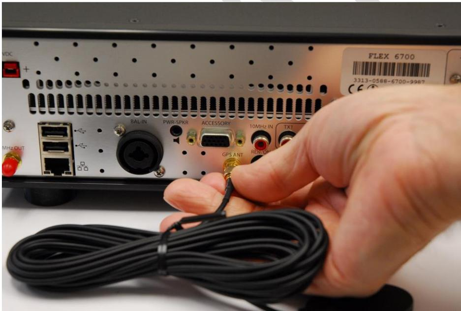
Using the double-sided adhesive oval that was included with the patch antenna, mount the GPS patch antenna on a window with a good view of the horizon.
