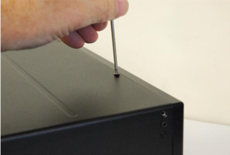
Once the bottom cover retaining screws have been removed, gently pull the Bottom Cover upwards to remove it from the FLEX-6000. The image below shows the removal of the Bottom Cover.
