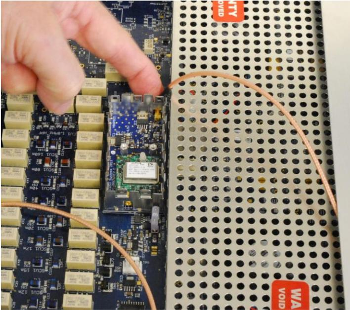
Press the **GPS ANT** coax assembly onto the MMCX connector on the GPSDO assembly module that faces the *back* of the FLEX-6000 as shown below.
