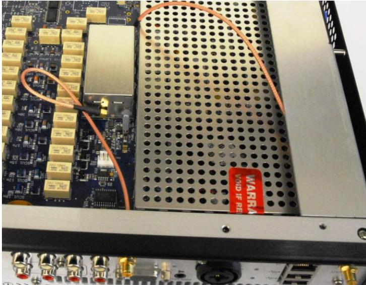
Orient the coax assemblies as show above, lying flat as possible. While holding the coax assembly in one hand, use either a 5/16" (4mm) open-ended wrench, socket or nut driver to slightly tighten the SMA connector hex nut to prevent the SMA connector from rotating as shown below.
