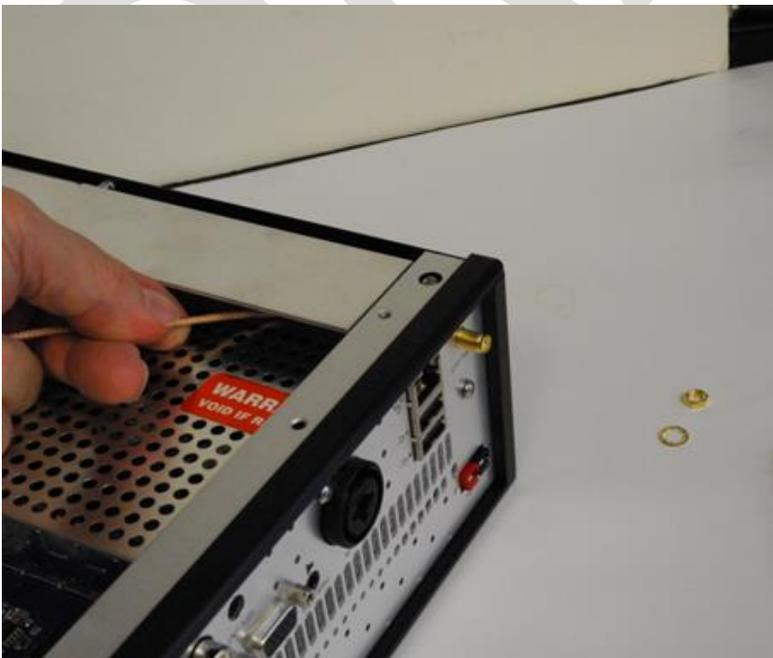
While firmly holding the long cable assembly in place with one hand, insert the lock washer on the threaded SMA connector. Carefully install the SMA connector 5/16" (8 mm) hex nut on the threaded SMA connector being careful not to cross thread the SMA connector. Tighten hex nut with your fingers so that the coax cable assembly will freely rotate.
