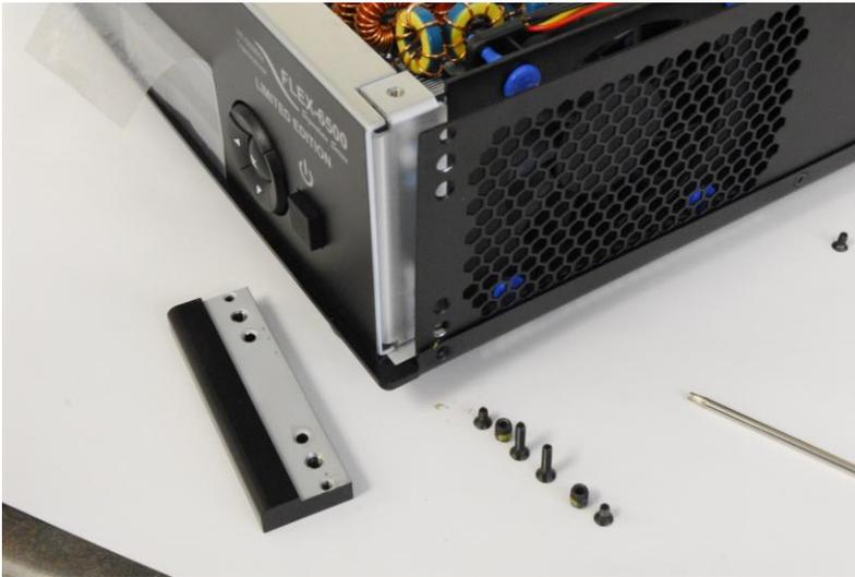
Remove the left front Frame Bezel after the right side front Frame Bezel has been removed.
