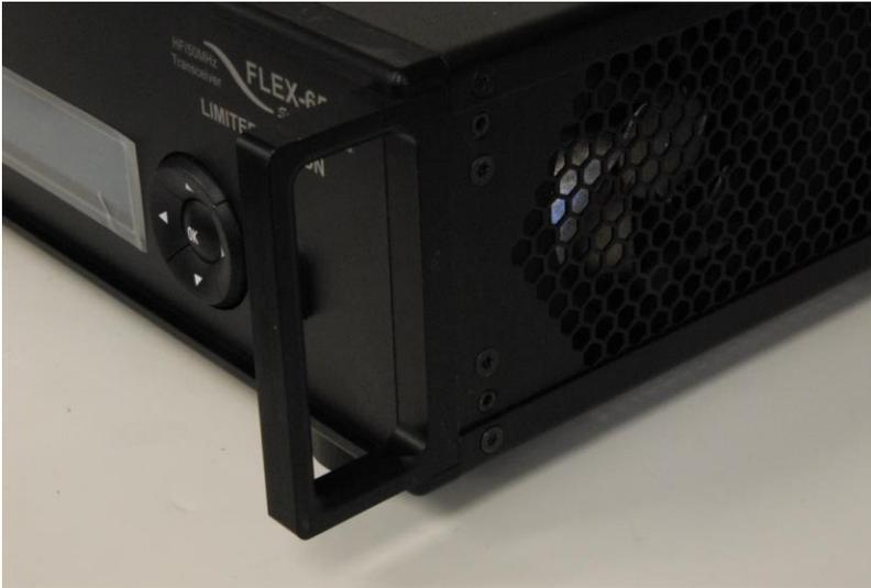
Re-install the side Cover and Set screws on the left side of the FLEX-6000 as described above. Once completed the radio should look like the image shown below.
