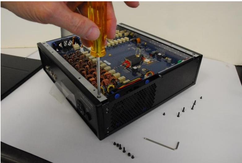
After both Front Chassis Retaining Bar screws have been removed, gently pull upward on the Front Chassis Retaining Bar to remove it from the chassis. Retain the Front Chassis Retaining Bar for re-installation. The image below shows the Front Chassis Retaining Bar being removed.
