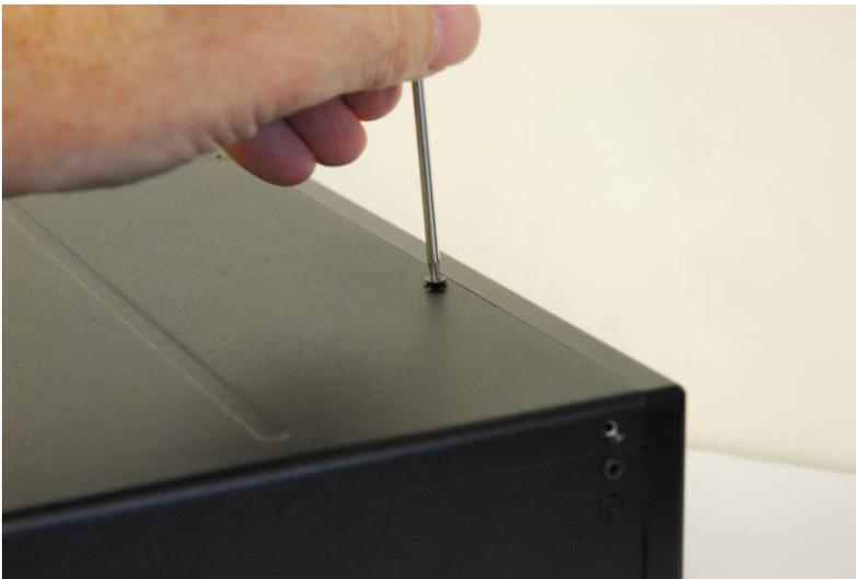
After replacing the four (4) long Top Cover screws, re-install two (2) short **Top Cover Side screws** on the left side of the FLEX-6000 in the middle and rear positions. Then re-install the two (2) short Top Cover Side screws from the right side of the FLEX-6000 in the middle and rear positions. *Do not over tighten the Top Side Cover screws.* The image below shows the re-installation of the middle right side top Cover Side screws.
