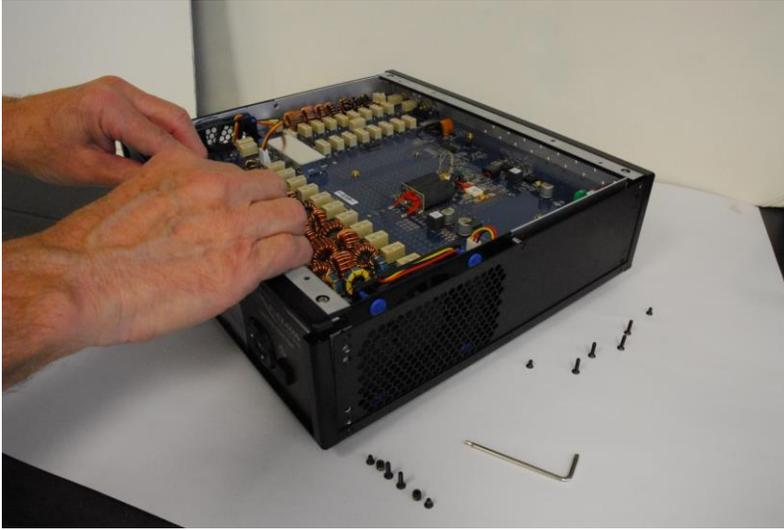
The image below shows the FLEX-6000 chassis with the Front Chassis Retaining Bar removed making it ready to remove the corner Frame Bezels. Be very careful not to disturb the PA inductor coils during the Front Chassis Retaining Bar removal.
