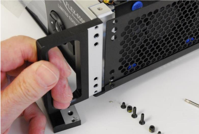
Repeat the procedure for the left handle. The image below shows both Handle Assemblies installed.
