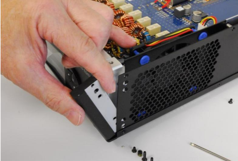
The image below shows the right front Frame Bezel after removal.
