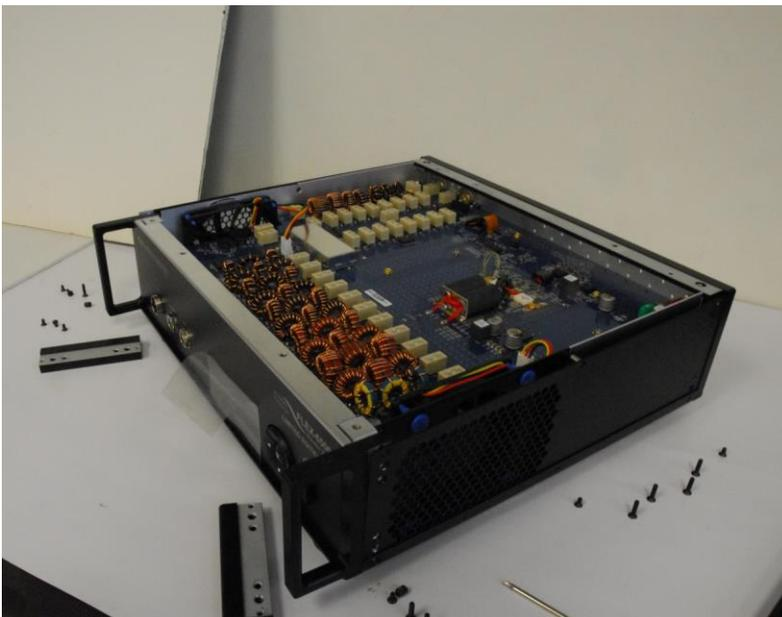
Reinstall the **Front Chassis Retaining Bar** by placing on top of the radio with the black edge facing outward and aligning the screw holes with the chassis holes. Install a chassis retaining bar screw and washer. Do not tighten the screw at this time. The image below shows the installation of right side chassis retaining bar screw.
