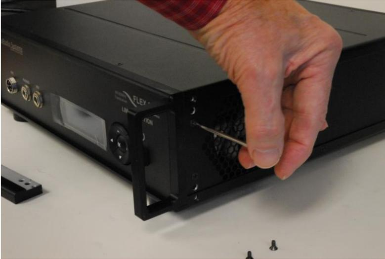
After removing the Set, Cover and Side plate screws, the corner of your FLEX-6000 should look like the image below.
