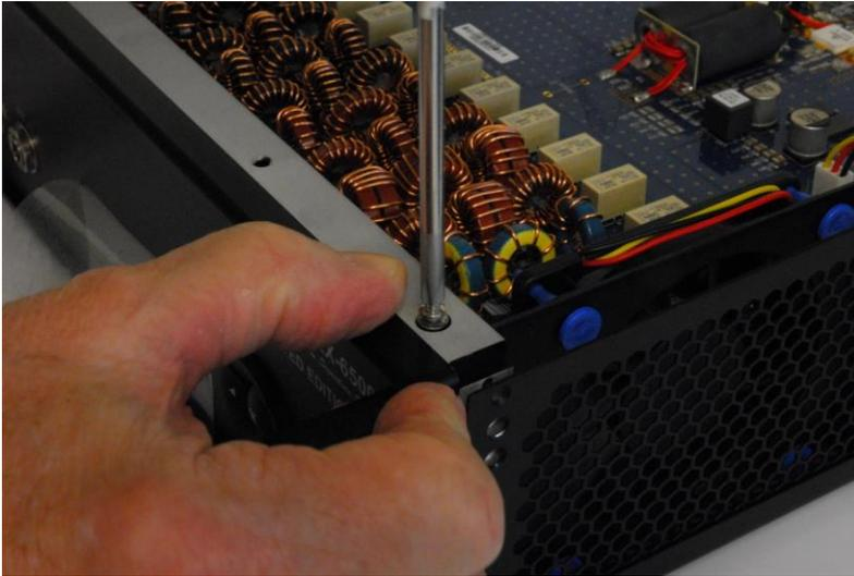
Install the left side chassis retaining bar screw and washer after the right side chassis retaining bar screw has been installed. Making sure that the holes in the Handle Assembly are aligned with the chassis holes, tighten the chassis retaining bar screws to hold the Handle Assembly in place. The image below shows the tightening of the left chassis retaining bar screw.
