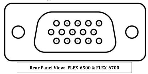
The accessory connector is a high-density HD-15 female connector. (This is the same connector used by VGA monitors.) There are a number of inputs and outputs on this connector.
