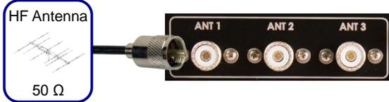
If you have the optional Antenna Tuner Installed, the impedance may deviate from 50 Ohm (see the Owner's Manual)
