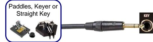
For paddles or a keyer, connect the Tip to DOT, Ring to DASH and Sleeve to common. For a straight key, connect Tip to KEY and Sleeve to common. Do not connect the Ring.
