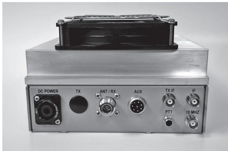
Figure 3: Rear panel of DEMI L432-28HP transverter
