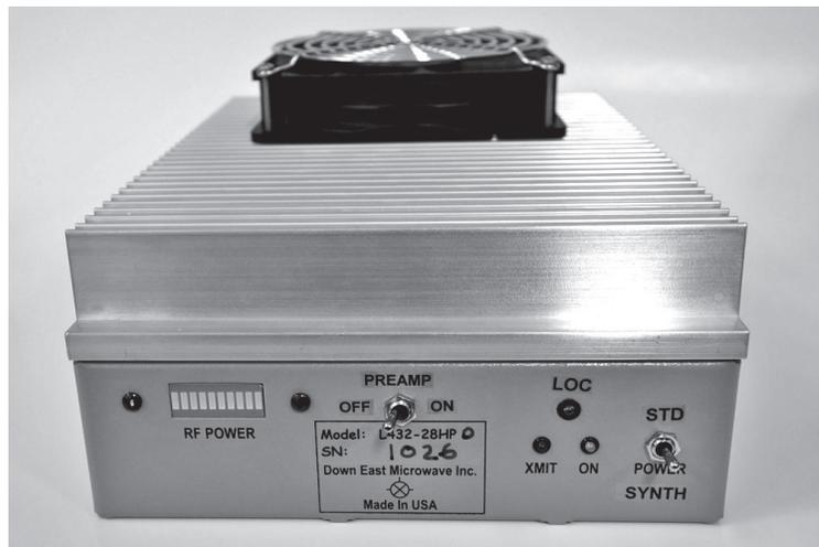
Figure 2: Front panel of DEMI L432-28HP transverter
