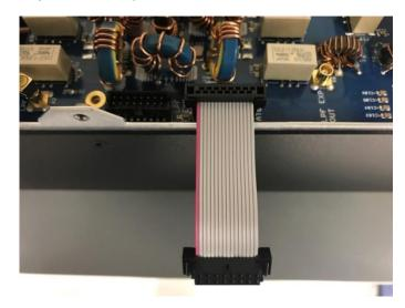
**Step 9:** Connect other end of ribbon cable to connection point on the ATU board.
