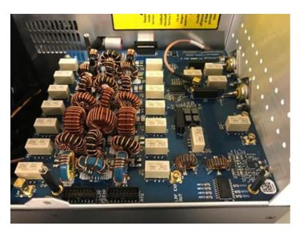
**Step 6:** Remove ATU from bag and insert the two cables provided as shown. Both cables should be inserted from the top with the straight connector going through the grommet and the right-angle connector on top. The longer of the two cables goes through the grommet nearest the inductors with the most coils.
