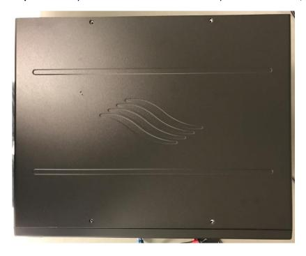
Step 2: Carefully remove screws (5 each side) from both sides of the top cover using the T8 Torx.
