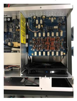
**Step 5:** Where the 3 screws were removed above, replace with the 3 stand offs included in the kit as show below. Two closest to board edge of the radio and one to the top left of the board.
