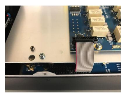
**Step 10:** Next set plate with ATU board down on the stand offs and align with the 3 screw holes.
