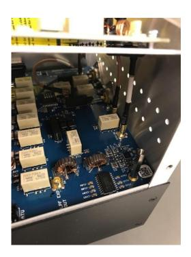
**Step 8:** Next, snap the ribbon cable to the connector on the bottom board as shown.
