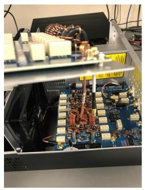
**Step 7:** Connect the coax to the board below by pressing until you hear it "click" into place. Repeat this process with the shorter coax by snapping into place as shown below. The longer coax goes in X10, ATU-OUT and the shorter coax goes into X9, ATU-IN
