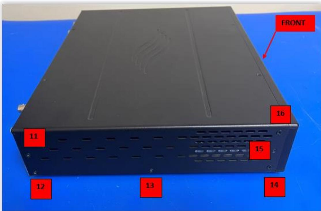
Once the top cover retaining screws have been removed, gently pull the top cover upwards to remove it from the FLEX-6000. The image below shows the removal of the top cover.
