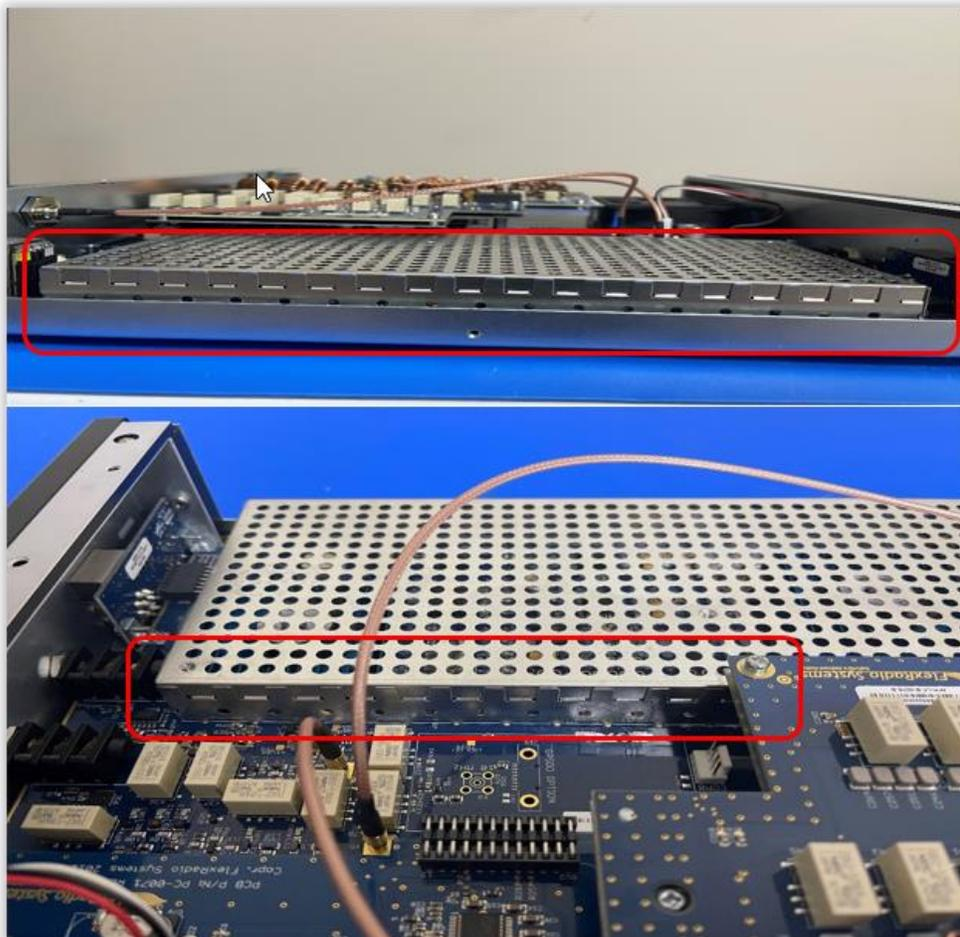
Replace the RF top cover and the 2 screws 17,18 with a Philips #1 screwdriver (Note: make sure the cage top cover is seated properly on all the 4 corners)
