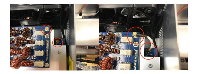
**Step 9:** Remove plastic insert from X3 connector of EXT TX. Connect the ribbon cable included in the kit to the X3 connector on the LPF board below first, then connect to the X3 connector of EXT TX board above.
