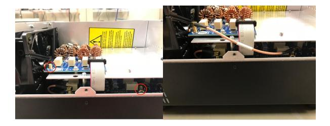
**Step 11:** Replace the top cover being careful to not pinch the coax cable and screw it into place using 4 screws in the top cover and 5 screws on each side.
