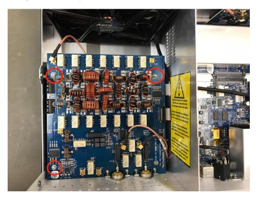
**Step 5:** Where the 3 screws were removed above, replace them with the 3 stand-offs included in the kit as shown below and tighten with a 3/16<sup>th</sup> hex driver.
